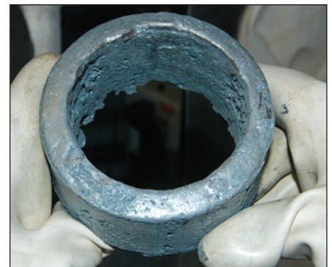
The final product: a ring of high-purity plutonium metal. The ring will be broken into pieces with a sample breaking press, and a small sample of one piece will be analyzed for purity. The remainder of the pieces will be stored under inert atmosphere to keep the plutonium from oxidizing.
